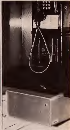
Text telephones , like this one found in Keller Conference Center, remain unobtrusive until activated by code. Once active, the silver box below the phone opens up to reveal a screen that allows hearing impaired individuals to see their conversations.
